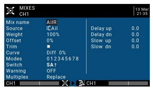
Mix name: Name setting Use the scroll wheel to select letters and numbers, and press and hold the ENT key to switch between upper and lower case. Short press the ENT key to set the next character.
