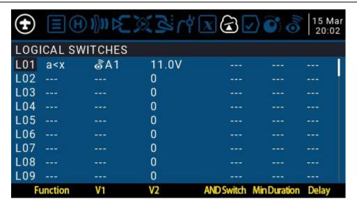
The setting of the LO1 example in the figure is expressed as follows: When the return value A1 is less than 11.0V, the LO1 switch is automatically turned on. In the settings of other pages, LO1 has the same function as the physical switch. You can define the corresponding function for LO1 on or off. In this way, a switch is automatically executed according to the parameters that change in real time.
