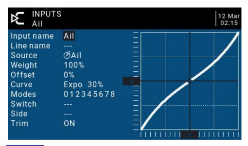
Input name: Name of the current entry. Use the scroll wheel to select a letter or number. Press and hold the ENT key to switch between upper and lower case. Press the ENT key to switch to the next character.
