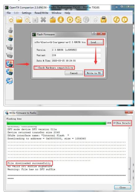
At this point, the firmware of the remote control is successfully written. Unplug the USB-C (TYPE-C) and proceed to the first boot procedures.
