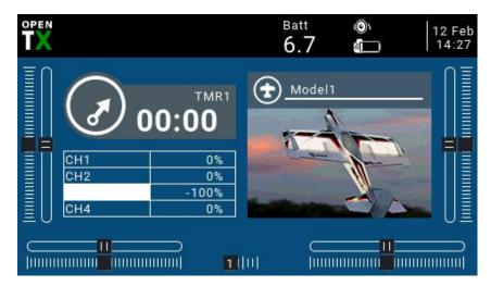
Top menu bar: The default top menu bar displays speaker volume, remote control battery level, receiver signal strength (RSSI), and time and date. Batt is a custom top display remote control voltage; users can also add other display information and widgets.
